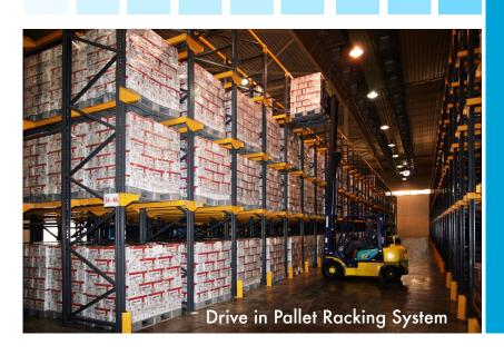
As it developed and evolved, Juhayna started facing problems such as storing capacity. That's when Linkmisr recommended the installation of the **Drive-in Pallet Racking**, which effectively provides a high density and extremely space efficient bulk storage system by using the minimum space for access aisles and lanes. However, with increased production rates at Juhayna, the high turnover remained a problem needing an appropriate solution given the existing warehouse heights.
