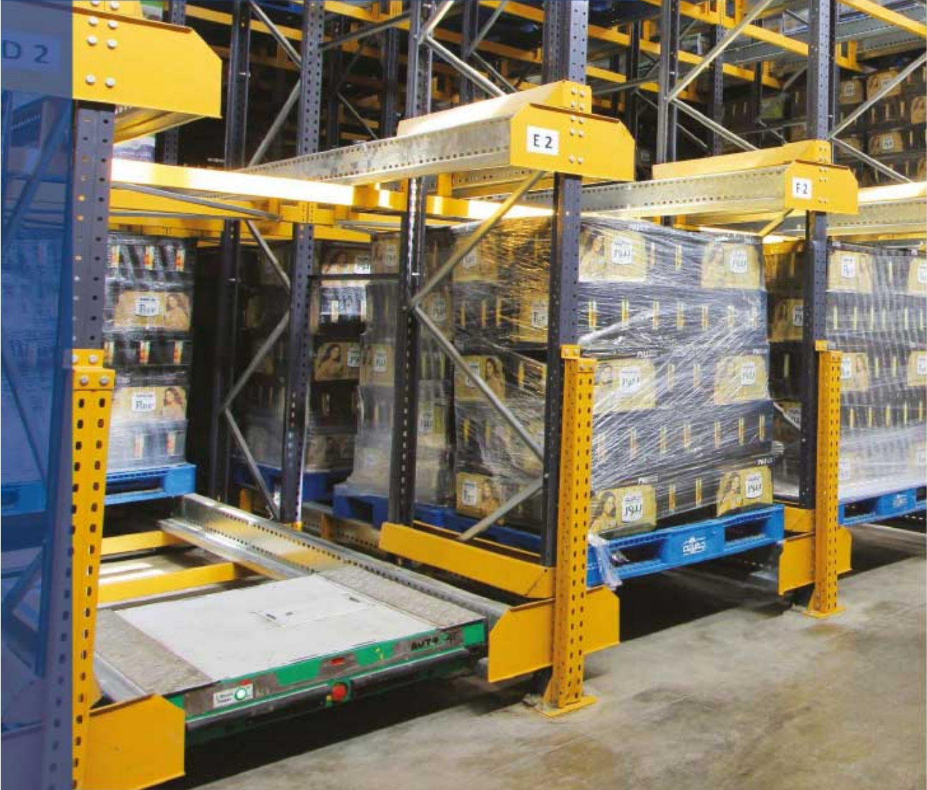
Satellite Storage System
